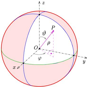
$$x = \rho \sin(\vartheta) \cos(\varphi), \quad y = \rho \sin(\vartheta) \sin(\varphi), \quad z = \rho \cos(\vartheta), \quad (10)$$
