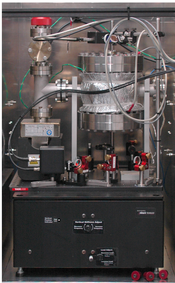
Figure 4.8.: Picture of the vacuum chamber containing the high-finesse cavity. The whole set-up is resting on a passive vibration-damping platform and is surrounded by a temperature-stabilized aluminum box.
