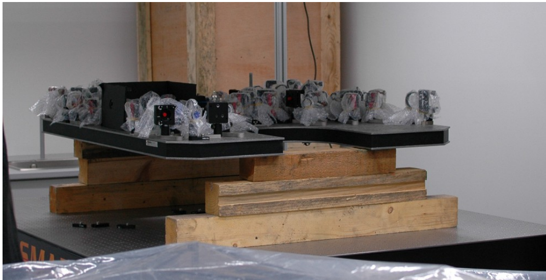
Figure 7.2.: Picture of trap table at the first day of the rebuilding phase in Saarbrücken (09/09/2010), trying a new sustainable ultra-stable mounting option for breadboards. A picture of the table after finishing the reconstruction is given in Figure 1.6.
