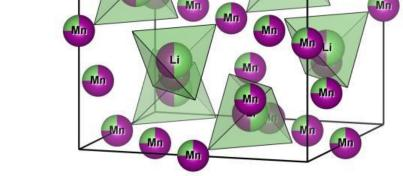
Disordered spinel structure of LiMn<sub>2</sub>O<sub>4</sub>
