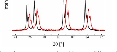
Section from a powder X-ray diffraction Pattern of partially delitiated  $LiMn_2O_4$
