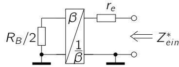
$$\begin{aligned}\frac{U_1}{I_1} &= R_E \parallel (R_T + Z_{ein}^*) \\ &= R_E \parallel (R_T + r_e + R_B/2\beta)\end{aligned}$$
