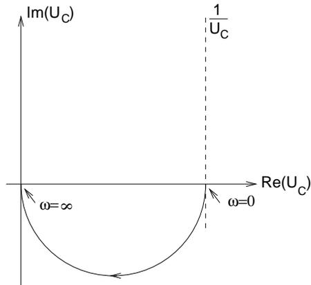
$$\begin{aligned} U_R &= U_2 \cdot \frac{R_2}{R_2 + j\omega L_2 + \frac{1}{j\omega C_2}} \\ &= U_2 \cdot \frac{R_2}{R_2 + j\left(\omega L_2 - \frac{1}{\omega C_2}\right)} \\ &= U_2 \cdot \frac{1}{1 + j\left(\omega \frac{L_2}{R_2} - \frac{1}{\omega R_2 C_2}\right)} \end{aligned}$$
