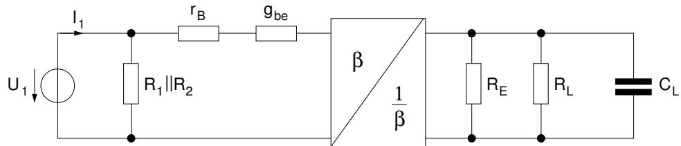
$$Z_{ein} = (R_1 || R_2) || \left( r_B + g_{be} + \beta \cdot \left( R_E || R_L || \frac{1}{j\omega C} \right) \right)$$
