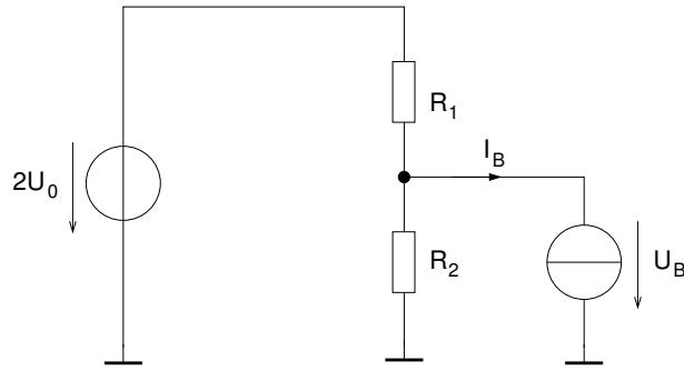
$$\begin{aligned} U_B &= \frac{R_2}{R_1 + R_2} \cdot 2U_0 - I_B (R_1 || R_2) \\ U_{BE} + U_0 &= \frac{R_2}{R_1 + R_2} \cdot 2U_0 - I_B (R_1 || R_2) \\ I_B &= \frac{I_E}{B+1} = \frac{\frac{U_0}{R_E}}{B+1} \\ \Rightarrow U_{BE} + U_0 &= \frac{R-2}{R_1 + R-2} \cdot 2U_0 - \frac{U_0}{B+1} \cdot \frac{R_1 R_2}{(R_1 + R_2) \cdot R_E} \end{aligned}$$
