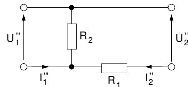
$$Y''_{11} = \left. \frac{I''_1}{U''_1} \right|_{U''_2=0} = \frac{1}{R_1} + \frac{1}{R_2}$$
