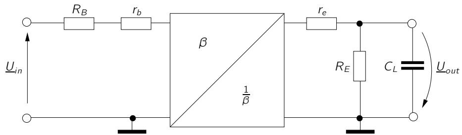
$$\begin{aligned} \frac{U_{out}}{U_{in}} &= - \frac{R_E \parallel \frac{1}{j\omega C_L}}{R_E \parallel \frac{1}{j\omega C_L} + \frac{1}{\beta} \left( \frac{1}{g_{be}} + r_b + R_B \right)} \\ &= - \frac{R_E}{R_E + j\omega C_L \left( R_E + \frac{1}{j\omega C_L} \right) \cdot \frac{1}{\beta} \left( \frac{1}{g_{be}} + r_b + R_B \right)} \end{aligned}$$
