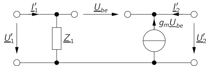
$$Y'_{11} = \left. \frac{\underline{I}'_1}{\underline{U}'_1} \right|_{\underline{U}'_2=0} = \frac{1}{Z_1} \quad Y'_{12} = \left. \frac{\underline{I}'_1}{\underline{U}'_2} \right|_{\underline{U}'_1=0} = 0$$
