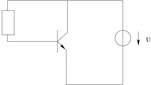
$$I_C = I_S e^{\frac{U_{BE}}{U_T}}, \quad I_C = 10mA, \quad I_S = 10^{-15}A$$
