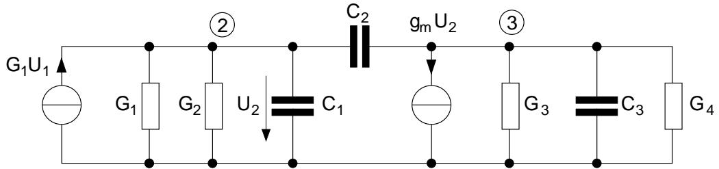
$$\begin{pmatrix} \underbrace{G_1 + G_2 + j\omega C_1 + j\omega C_2}_{k_1} & -j\omega C_2 \\ -j\omega C_2 + g_m & \underbrace{j\omega C_2 + G_3 + j\omega C_3 + G_4}_{k_2} \end{pmatrix} \begin{pmatrix} \underline{U}_2 \\ \underline{U}_3 \end{pmatrix} = \begin{pmatrix} \underline{U}_1 G_1 \\ 0 \end{pmatrix}$$
