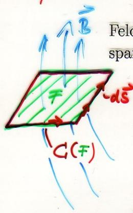
$$\iint_F \text{rot } \vec{E} d\vec{f} = -\iint_F \frac{\partial \vec{B}}{\partial t} d\vec{f} = -\frac{\partial}{\partial t} \iint_F \vec{B} d\vec{f} = -\frac{\partial \phi}{\partial t} \quad (7)$$
