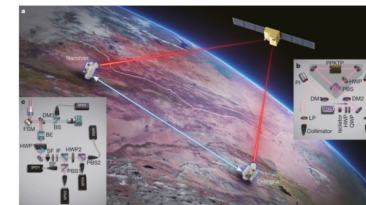
Fig. 1: Overview of the experimental set-up of entanglement based quantum key distribution.
