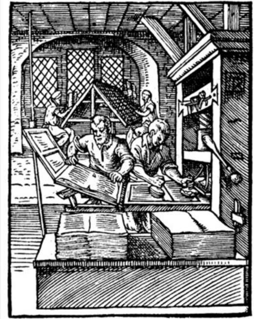
Early wooden printing press, depicted in 1568. Such presses could produce up to 240 impressions per hour. [16]
