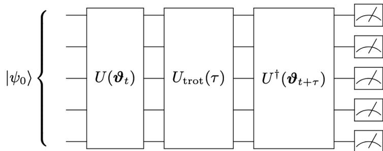
Return probability to initial state is maximal for optimal parameters  $\vartheta_{t+\tau}$
