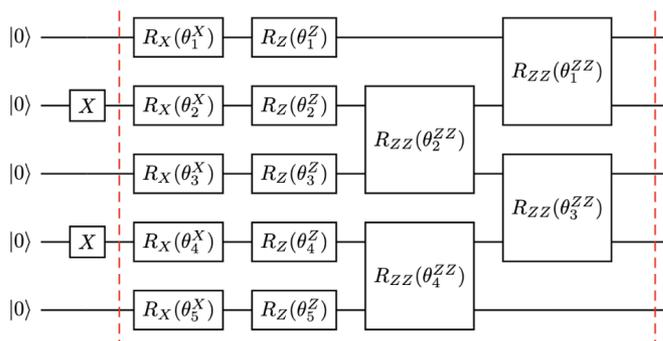
One step of Trotter circuit in L=5 system, starting from Neel state.
