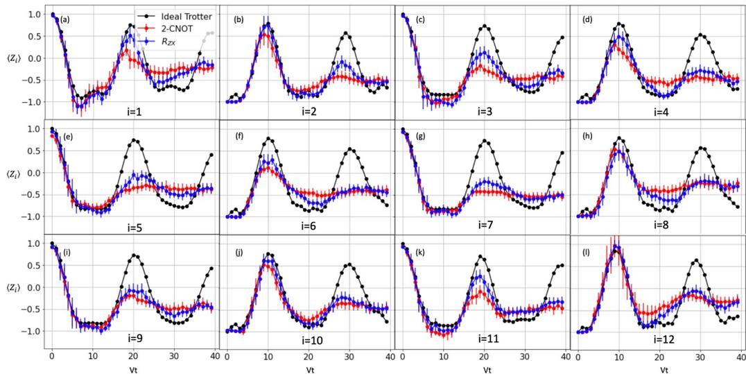
FIG. 11. Complete list of error-mitigated local magnetization results  $\langle Z_i \rangle$  versus time  $Vt$  for a 12-site chain measured on `ibmq_guadelupe` using the scaled- $R_{ZX}$  and two-CNOT implementations (blue and red, respectively). The ideal Trotter simulation data (black) are also shown for reference.
