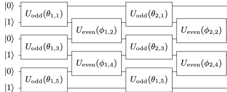
> Determine depth of layered ansatz  $\ell \equiv \ell^*$  to accurately describe  $|\psi(t)\rangle$
