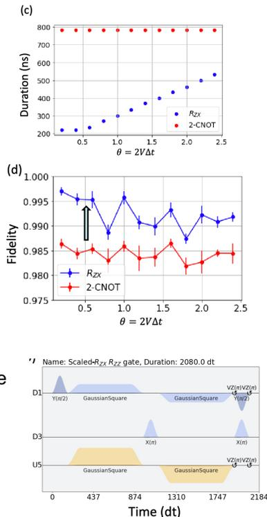
$V = 0.9, \Omega = 0.6$  ZNE used linear extrapolation and scale factors  $\{1, 1.5, 2\}$ .
