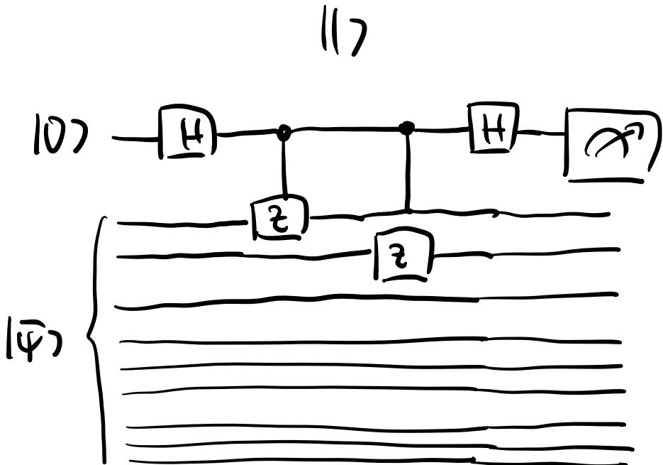
$$|0\rangle |\Psi\rangle \rightarrow \left( \frac{1}{\sqrt{2}} |0\rangle + |1\rangle \right) |\Psi\rangle \rightarrow \left( \frac{1}{\sqrt{2}} |0\rangle |\Psi\rangle + Z_1 Z_2 |1\rangle |\Psi\rangle \right)$$
